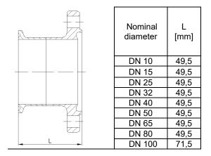
Threaded connection according to DIN 11851
